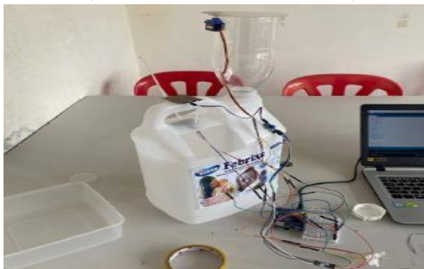
Figure 6: Rainwater Harvesting Prototype
