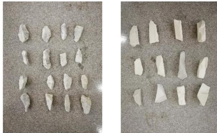
Figure 4.2: The aggregate samples (a) NA, (b) CTWA for the elongation index test
