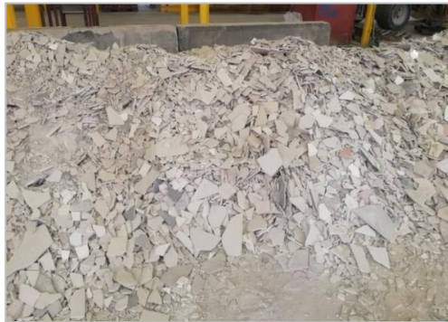
Figure 3.1: A stockpile of ceramic tile waste was used in the study
