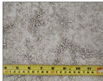
Figure 3.2: Crushed ceramic tile waste
