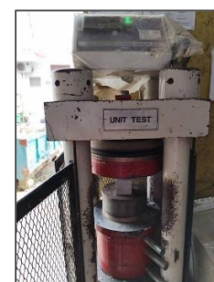
Figure 3.4: Compression strength test of cube specimens
