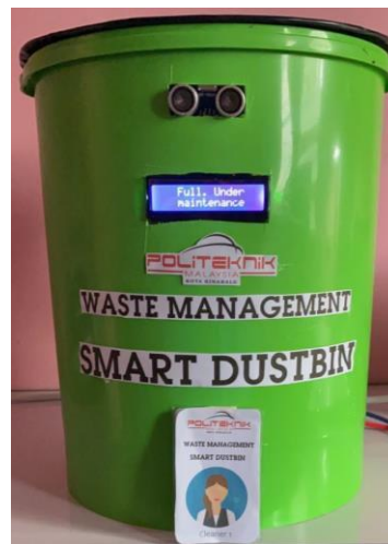
Fig. 6. Message display on the LCD when the Dustbin is full.
