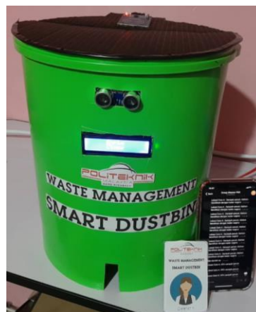
Fig. 7. Smart Dustbin with RFID Card and Smartphone notification
