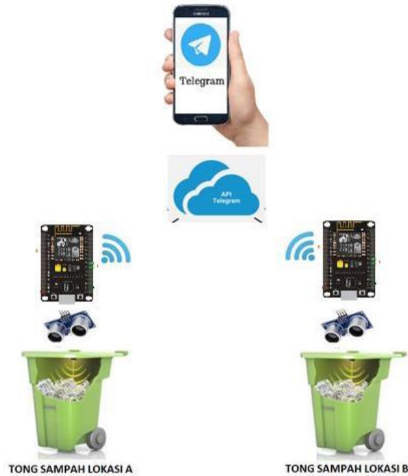
Fig. 4. Concept of notification system based on location.
