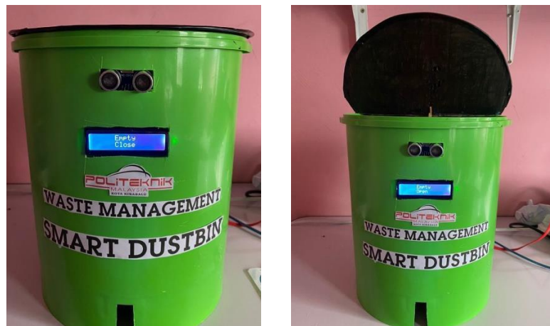
Fig. 3. Smart Dustbin when the dustbin lid open and close
