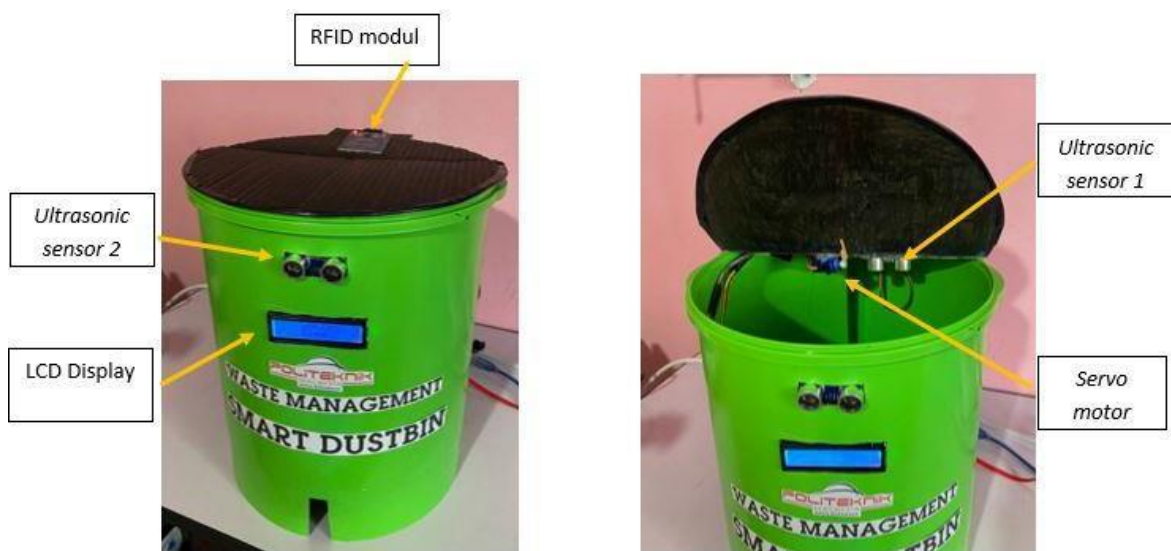
Fig. 2. Physical Prototype Design of Smart Dustbin
