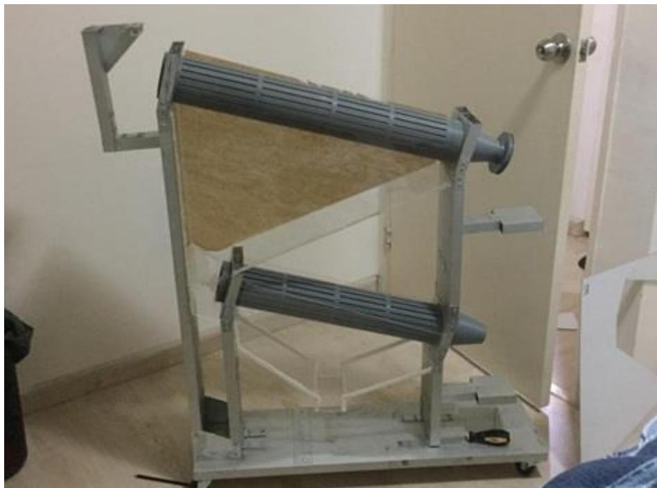
**Figure 4:** Aluminum frame structure part was fabricated by riveting to join each component
