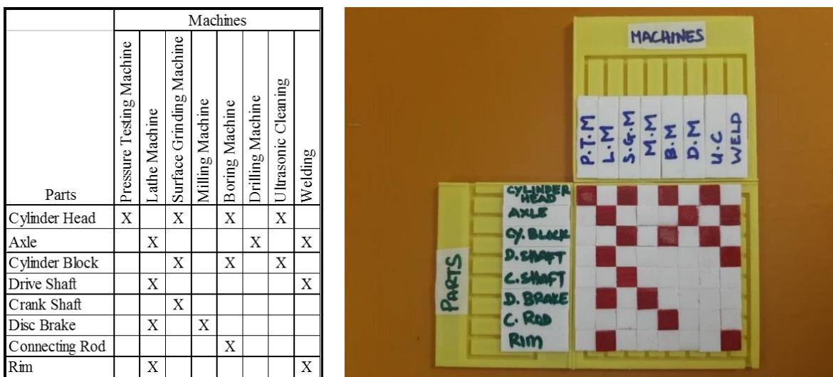
**Figure 5:** Parts and its operation sequences on paper (left) and aid tools (right).
