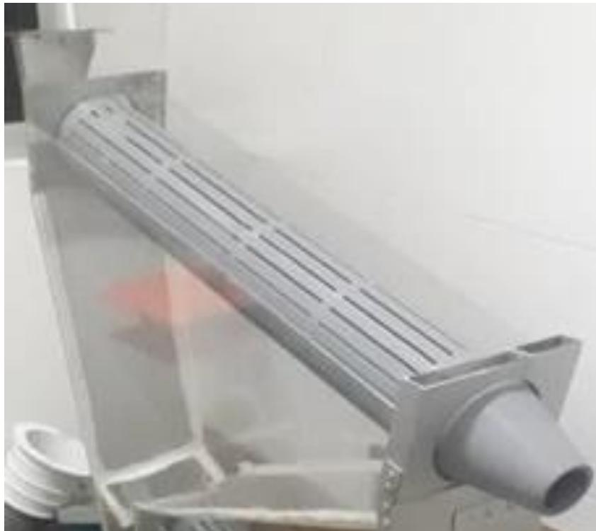
**Figure 3:** Filter housing part was built by using 3d printer technology
