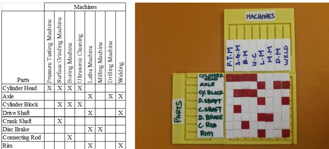
**Figure 6:** Reordering process by sorting machines on paper (left) and aid tools (right).
