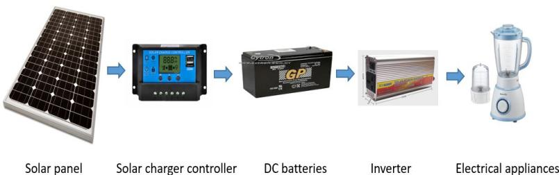
**Figure 3.1:** Flow process of solar generator
