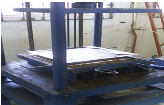
Figure 6.8: Stalk/skewer cold compaction.
