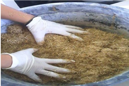
Figure 6.6: Oil palm stalk/skewer mixing with UF resin.
