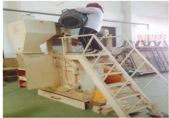
Figure 6.4: Oil palm stalk/skewer grinding process.
