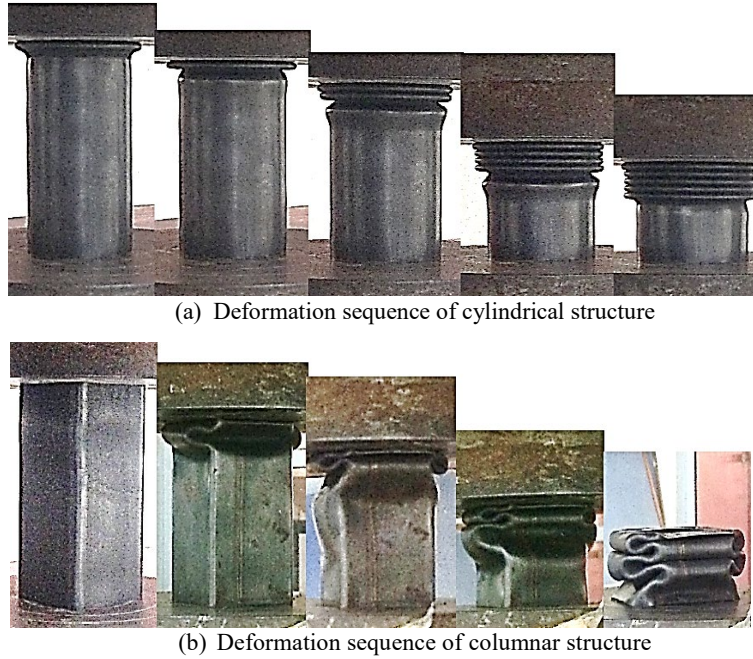
Figure 5: Crushing process mechanism
